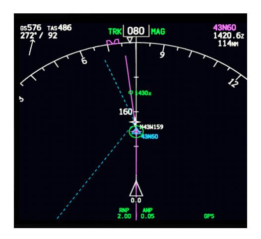
The ND showing RTE 1 legs. We are approaching 43N 160W, which concides with the ETOPS critical point for RJCC/PASY. It shows what the ETOPS set up does for us along the way in terms of situational awareness.
