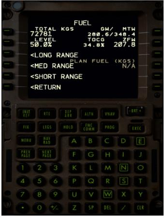
Get the zero fuel weight and fuel data from the OFP and load them in the FS Options section in the 777 FMC. The -200LR has quite the range so this 8-9 hour flight is more or less a walk in the park. Using the Export function on PFPX you should already have route and wind data available so you proceed with the usual set up, which we will briefly go over.
