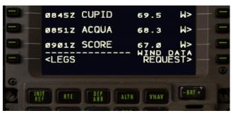
RTE DATA: It is a good time to fetch wind data now so that you have an actual estimate for the fuel remaining in SFO and make sure everything is OK. Wind data can be fetched from the LEGS / RTE DATA page. LSK6R (WIND DATA REQUEST) will load the data as exported by PFPX.
