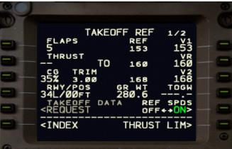
**TAKE OFF:** I skipped the THRUST LIM page because I left everything at the default setting with no derate. We are not about to get the take off speeds and the trim setting. Note the trim and speeds so you can configure properly the MCP as well as actually set the trim the calculated value for take off.
